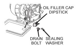
Figure 14. Engine Oil (Draining)
